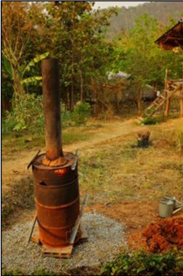
Gasifier biochar production system made from two 200 L drums and scrap metal. (Photo by Lyse Kong.)
