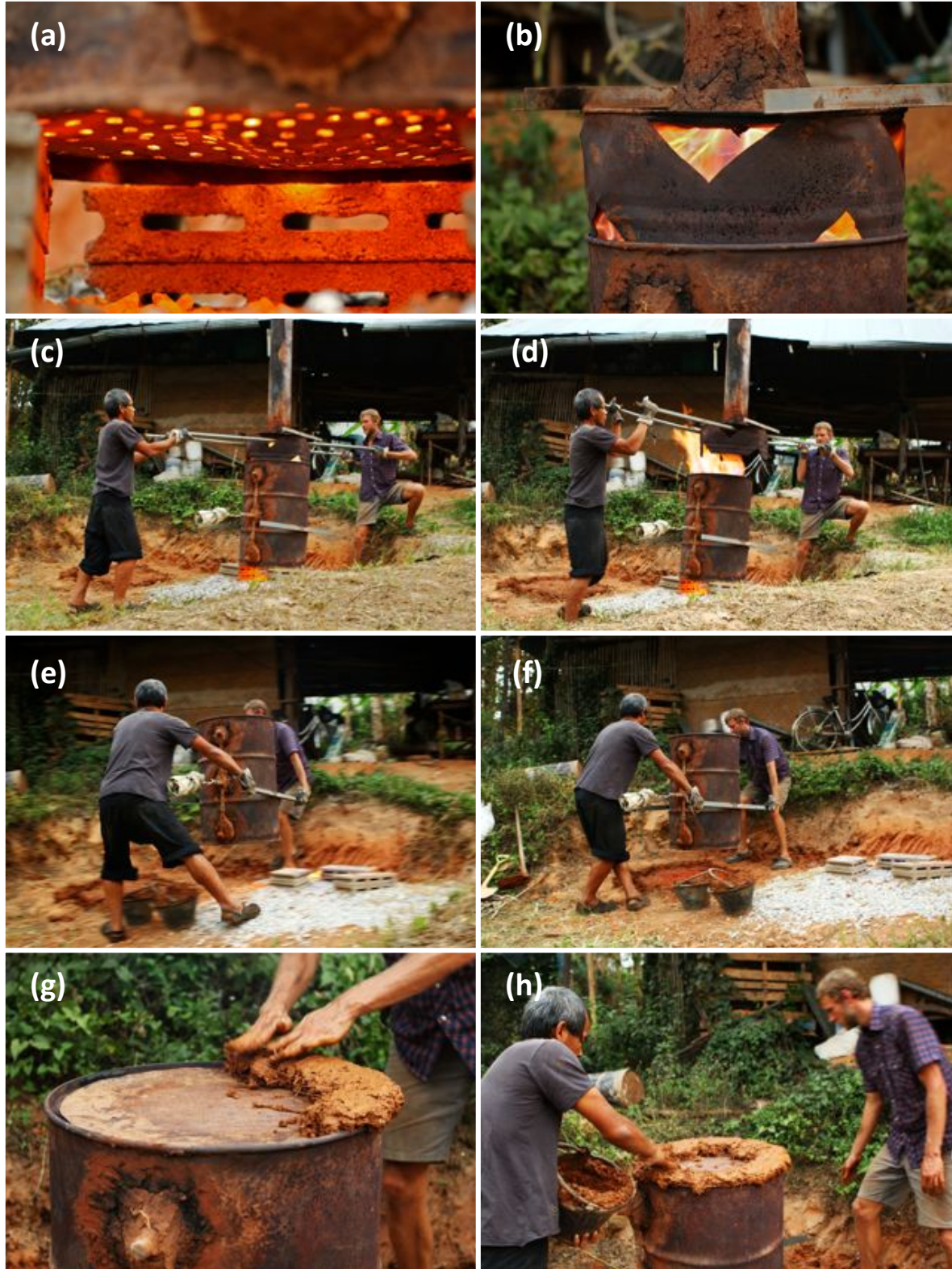
Photo series showing shutdown procedure: When bottom of drum begins to glow (a) and blue flames appear in crown (b) then pyrolysis is nearing completion. Remove the crown and chimney (c) and (d). Put on the lid and move the reactor body to the adjacent mud pit to seal the bottom (e) and (f). Seal the top with mud to prevent air leaks (g) and (h). (Photography by Lyse Kong.)
