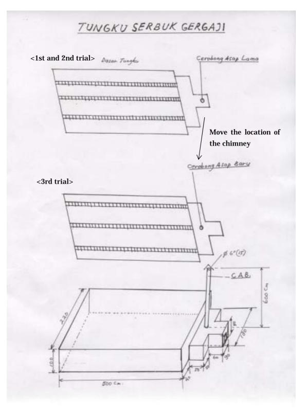
Fig.2 Description of a flat kiln
