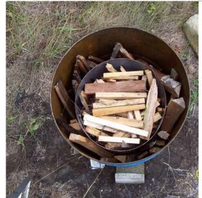
Fill center cylinder with wood for charcoal; space between cylinders with wood to burn.
