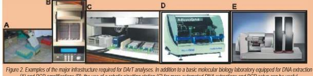
Figure 2. Examples of the major infrastructure required for DArT analyses. In addition to a basic molecular biology laboratory equipped for DNA extraction (A) and PCR amplifications (B), the use of a robotic pipetting station (C) for more automated DNA extractions and PCR setup can be useful. The two major pieces of equipment required are a microarrayer (D) to print the arrays contained the DArT markers and a scanner (E) to detect the signals following hybridization with sample DNA.
